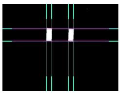
The vertical line groups were considered to be the edge of the target. Using a pixel to inches conversion value, we were able to compare the the target's width to the theoretical target's widths, in order to determine the angle of the robot. The angle of the incidence of the target and the distance from the target were also calculated based on these ratios.
