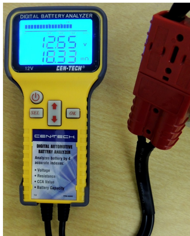
Figure 12 – Digital Battery Analyzer [9].
